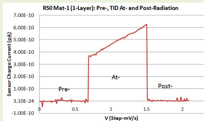
**Figure 6: The first material used for the sensor and results of pre-, at- 3.75-6.25E10pA and post- TID results as radiated in ionizing air environment of X-ray**
