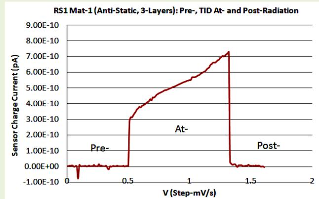
Figure 7: The second material used for the sensor with non-static coating and results of pre-, at 3.0-7.0E10pA and post- TID results as radiated in ionizing air environment of X-ray
