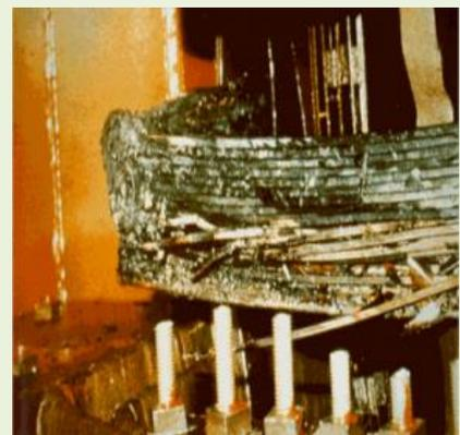
**Figure 5: Ruptured line-Power Transformer**
